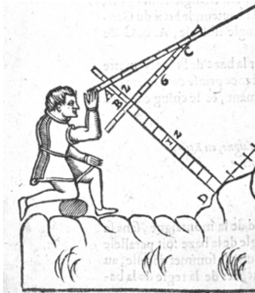
Fig. 4. A Henry-metre in use for measurement of height, from the woodcut illustration p. 80.
